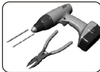
Cutting nipper, Electrical Drill &amp; Drilling bits
